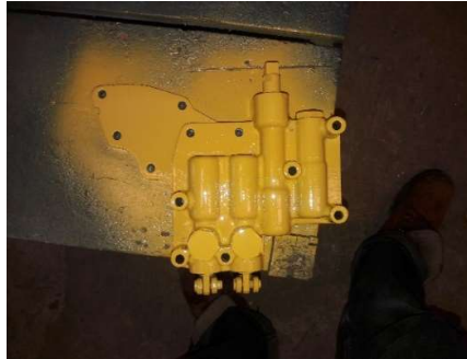
Gambar : 77. control valve
