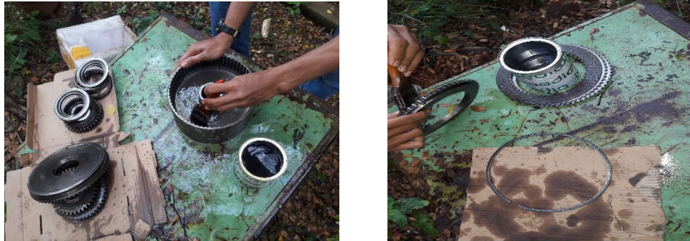
Gambar : 50. Proses pencucian komponen countershaft
