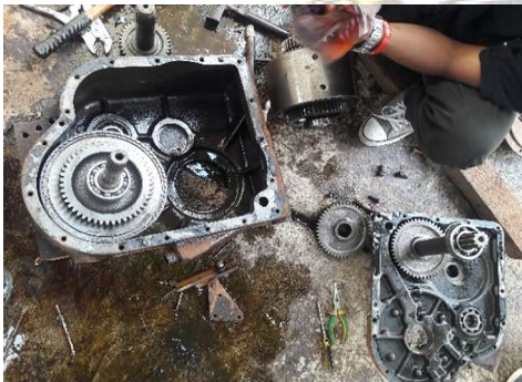
Gambar : 45. Proses pembongkaran countershaft dan housing countershaft
