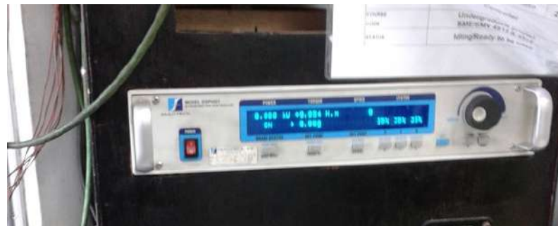
Figure 3.6 The 19" Magtrol DSP6001 Dynamometer Controller
