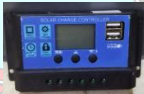
Gambar 2. 7 Solar Charger Control
