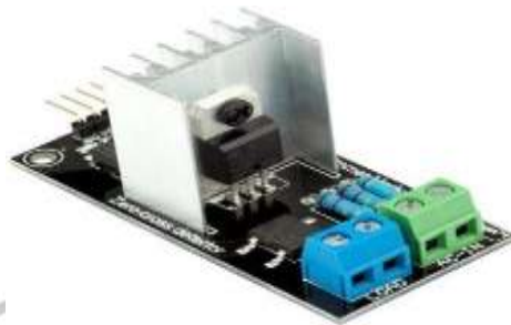
Gambar 2.4 Module Dimmer AC (Sumber: https://electroslab.com/products/ac-light-dimmer-module )
