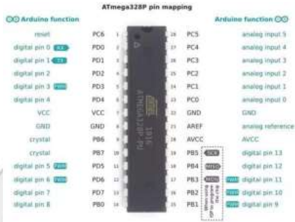
Gambar 2.2 Pin Mapping ATmega328P
