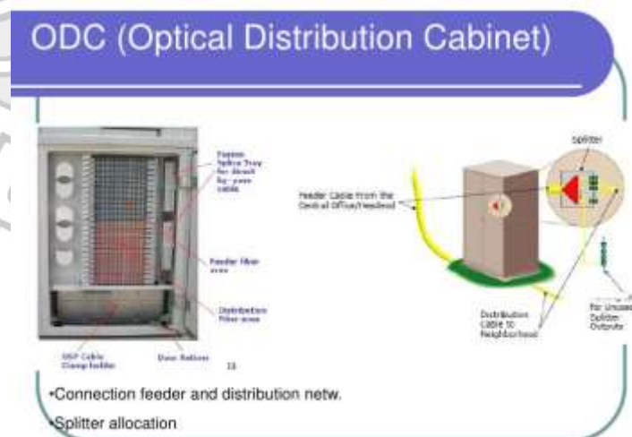
Gambar 2. 15 Optical Distribution Cabinet
