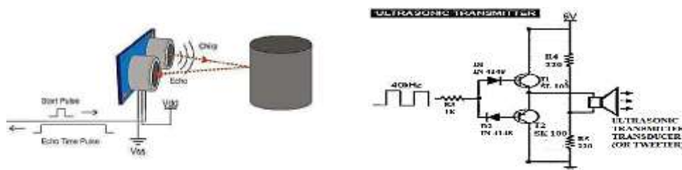
Figure 6. The working principle of an ultrasonic sensor
