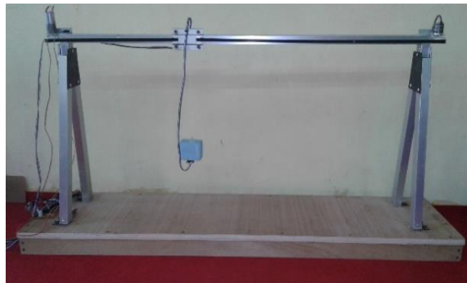
Figure 4. Experimental model of the gantry crane system
