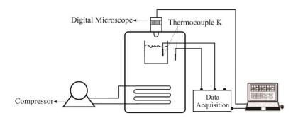
Fig. 1. Scheme of data acquisition morphological test.
