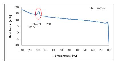
Fig. 3. The heat fusion of ricinoleic acid vs temperature.
