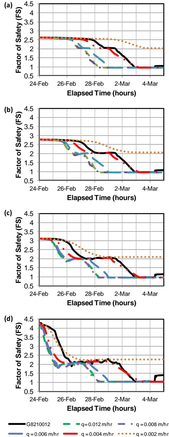
Figure 6 Variation of factor of safety with various rainfall intensity and failure plane at (a) 2 m depth, (b) 1.5 m depth, (c) 1 m depth, (d) 0.5 m depth.
