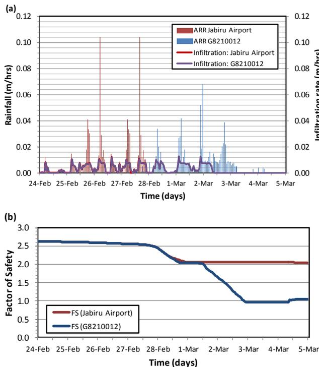
Figure 5 (a) Simulated infiltration, (b) Computed factor of safety with the elapsed time of rainfall on the failure-plane at 2 m depth below slope surface.
