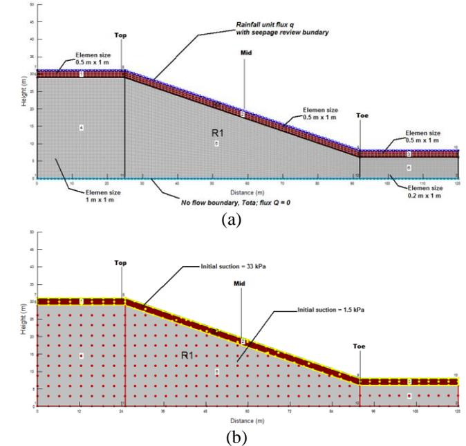
Figure 3 (a) Slope geometry and boundary conditions of the slope for transient analysis (b) Boundary conditions for generating initial pore-water pressure
