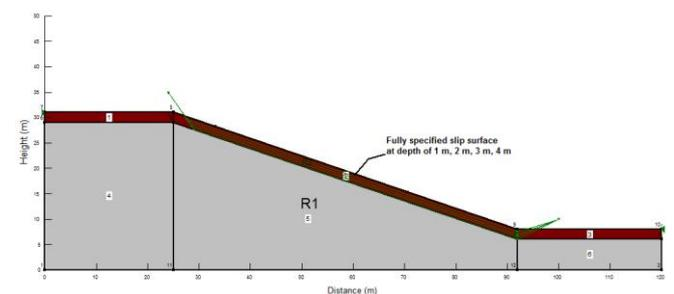
Figure 4 Range of possible critical slip surfaces used for the slope stability analysis
