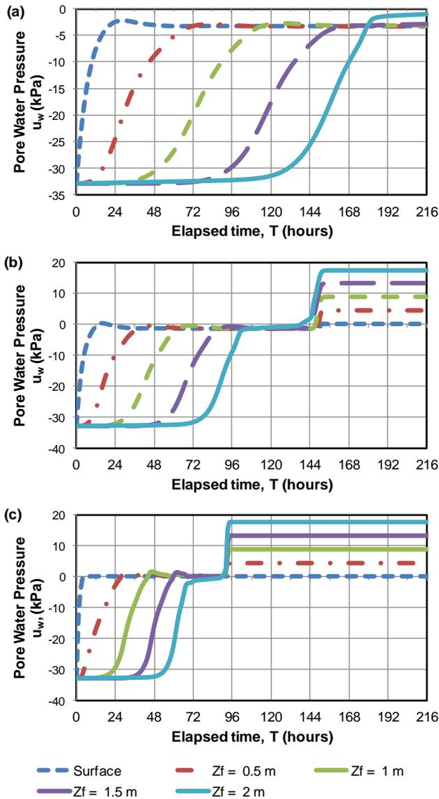
Figure 7 Variation of pore water pressure with the duration of rainfall (a)  $I = 0.002$  m/hr ( $I/k_{sat} = 0.25$ ), (b)  $I = 0.004$  m/hr ( $I/k_{sat} = 0.5$ ), (c)  $I = 0.012$  m/hr ( $I/k_{sat} = 1.5$ ).
