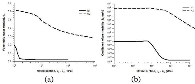
Figure 2 Soil-water characteristic curves and permeability functions with varying a values for the soils used in the study
