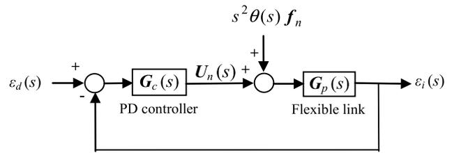
$\varepsilon_d$ : Desired strain,  $\varepsilon_i$ : Measured strains at Node  $i$
