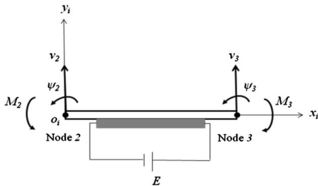
**Fig. 5** Modeling of piezoelectric actuator (top view)
