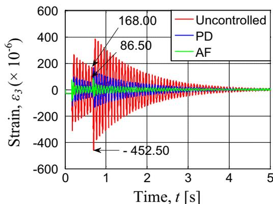
**Fig. 8** Calculated time history responses of strains at Node 3 for uncontrolled and controlled Model A due to the excitation force generated by the motor's rotation [ $K_p = 600$  (Nm),  $K_d = 0.005$  (Nms), and  $K_{pa} = 0.83$  (-)]
