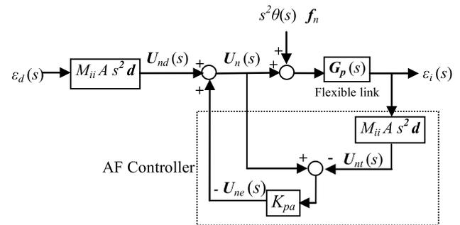
$\varepsilon_d$ : Desired strain,  $\varepsilon_i$ : Measured strains at Node  $i$
