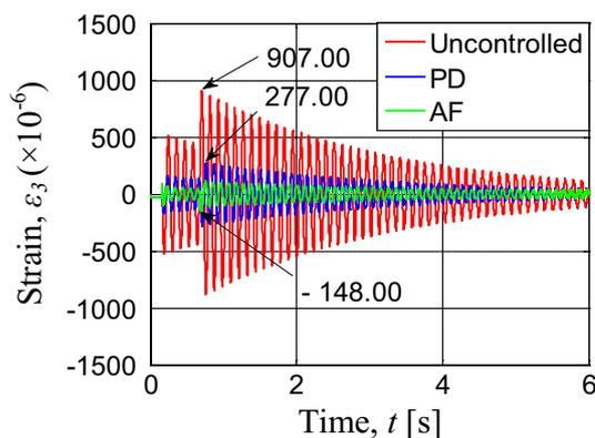
**Fig. 9** Calculated time history responses of strains at Node 3 for uncontrolled and controlled Model B due to the excitation force generated by the motor's rotation [ $m_c = 0.005$  (kg),  $K_p = 600$  (Nm),  $K_d = 0.005$  (Nms), and  $K_{pa} = 0.83$  (-)]
