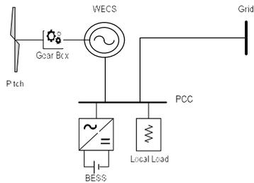
Figure 1. Typical configuration of a WECS-grid connected with BESS
