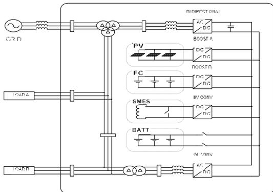
Figure 4. New type dispersed power system that uses SMES unit [31]
