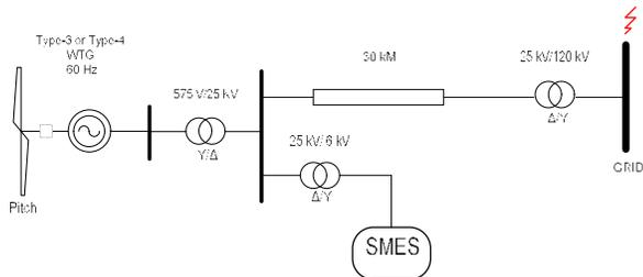
Figure 5. Application of SMES unit on variable speed WECS during grid disturbances [39]
