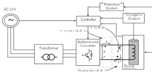
Figure 3. Typical schematic diagram of a SMES unit [28]
