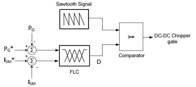
Fig. 7. Control algorithm of DC-DC chopper
