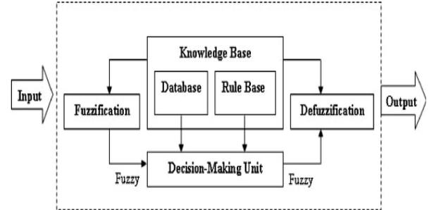
Fig. 8 Fuzzy logic model flow chart
