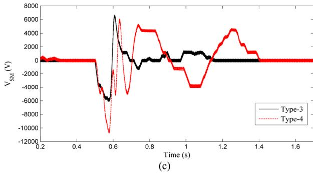
Fig. 15. SMES coil behavior during voltage sag: (a) Energy of SMES coil (b) Current of SMES coil and (c) Voltage across the SMES coil
