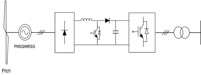
Fig. 2. Typical configuration of Type-4 WT
