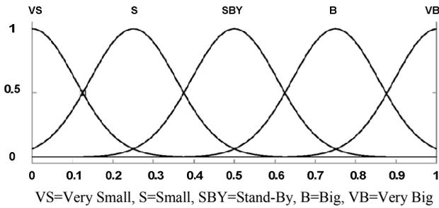
Fig. 11. Output variable MF – Duty cycle
