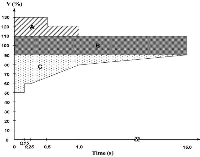
Fig. 3. Fault-Ride-Through of Spain grid code [5]
