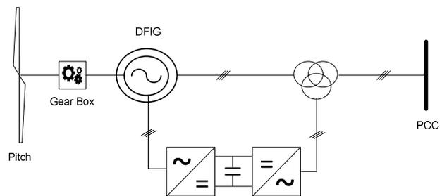
Fig. 1. Typical configuration Type-3 WT
