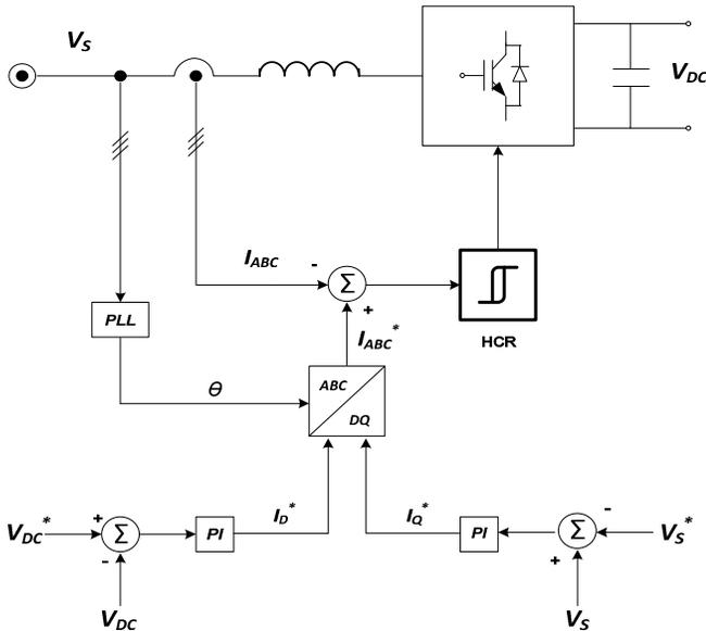
Fig. 6. Control algorithm of VSC
