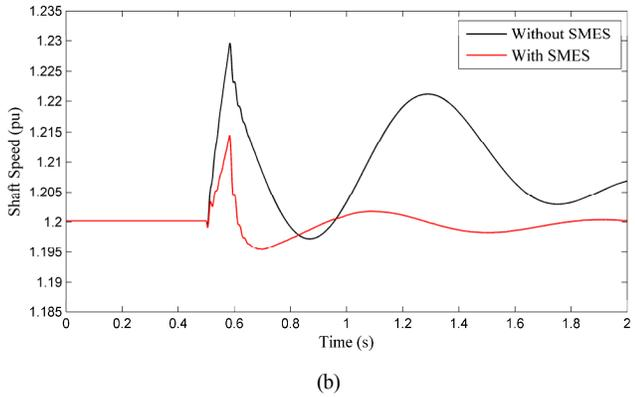
Fig. 13. Type-3 WTG response: (a)  $V_{DC}$  wave form (b) shaft speed response
