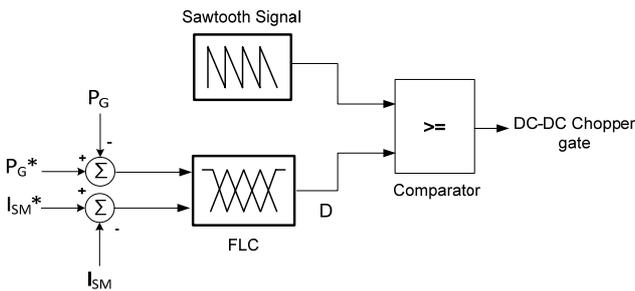
Figure 4: Control algorithm of DC-DC chopper
