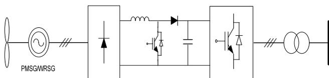
Figure 1: Typical configuration of type-4 WTG
