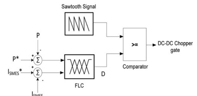
Fig. 5 Fuzzy logic control scheme
