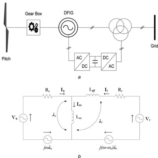
Fig. 1 DFIG equivalent circuit and system under study
