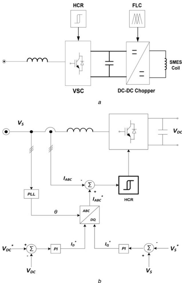
Fig. 4 Configuration of SMES and VSC control schemes
