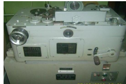
Gambar 5. Ogoshi high speed universal wear testing machine type OAT-U
