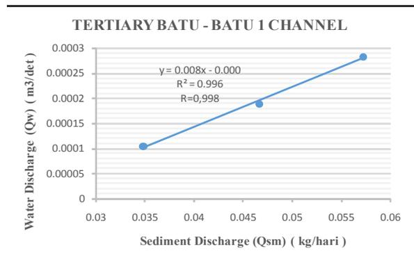
**Figure-8.** Relations sediment discharge and water discharge at the tertiary Batu-Batu 1 channel.
