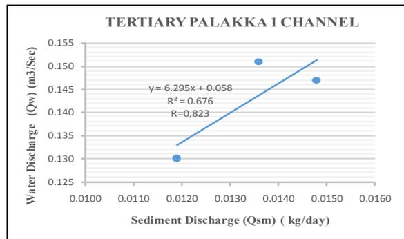
**Figure-6.** Relations sediment discharge and water discharge at the tertiary Palakka 1 Channel.
