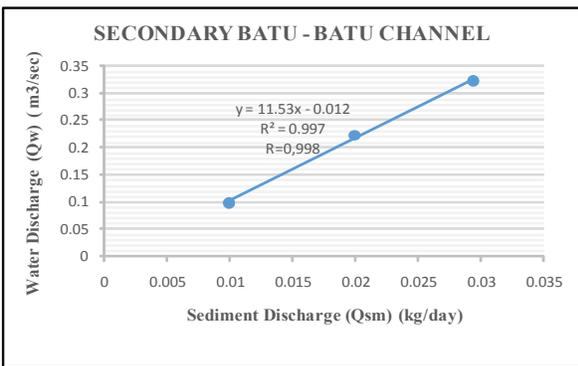
**Figure-5.** Relations sediment discharge and water discharge on the secondary Batu-Batu channel.
