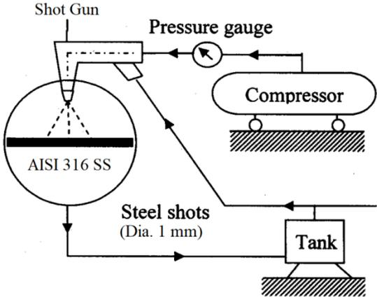
Figure 2. Schematic of the shot peening process
