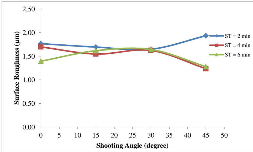
**Figure 3.** Data on surface roughness for different shooting time ( $S_T$ ).
