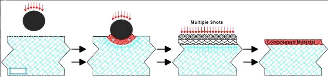
Figure 1. Illustration of shot peening
