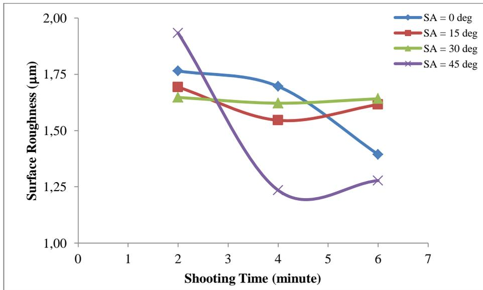
**Figure 4.** Data on surface roughness for different shooting angle ( $S_A$ ).
