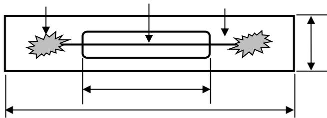
**Figure 1.** Specimen of single fiber test ASTM 3379-02 for tensile test.
