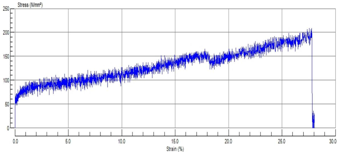
**Figure 3.** Stress and strain diagram for coconut fiber as result of UMT after treatment with NaOH 20% for one hour (1h).
